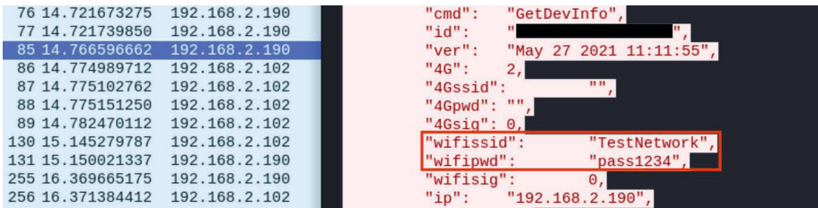
Fig. 3. Extracting Wi-Fi credentials in Wireshark
