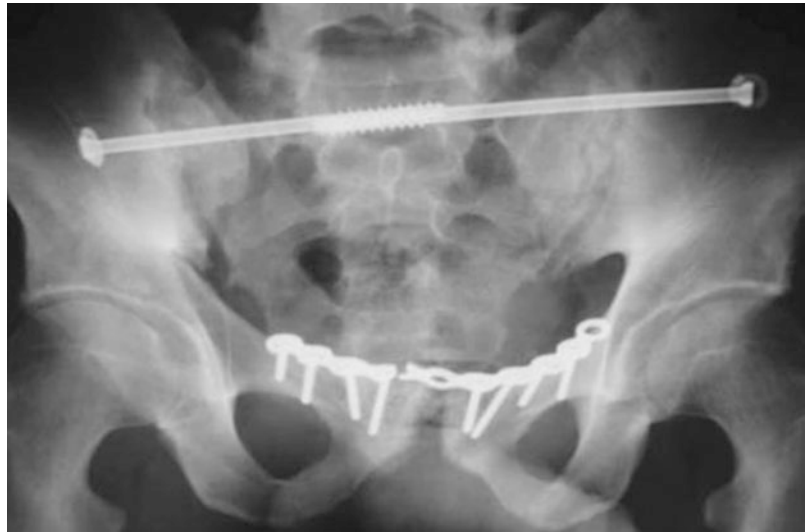
Fig. 1.2 Anteroposterior (AP) pelvic radiograph demonstrating a broken 3.5 mm matta plate. As a plate that spans the symphysis, this construct is continually exposed to bending stresses that lead to plate failure by fatigue (in this case the residual pubis diastasis that developed after failure of the plate did not require any further intervention as the patient was asymptomatic)
