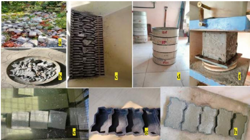
Fig. 2 a Building wastes, b hammered and collected in pan, c into the shredder, d sieving to correct grade sizes, e cube casted for strength tests, f compression testing, g interlock mold-zig-zag ant shape, h interlock block casted
