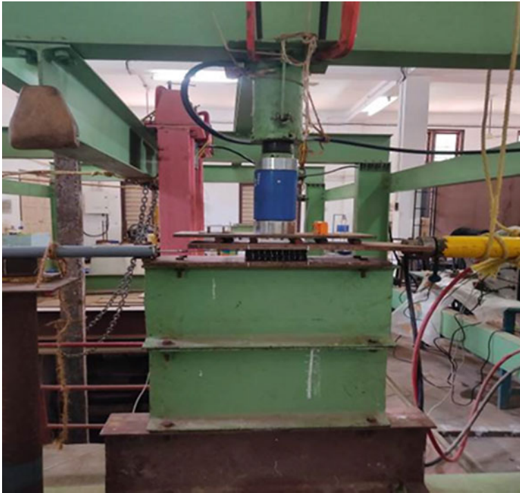
Fig. 4 Experimental Setup for cyclic loading
