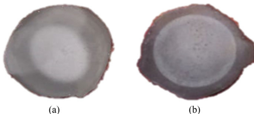
Fig. 2 Nital TM ring test results of collected samples with a Composition-1 and b Composition-2
