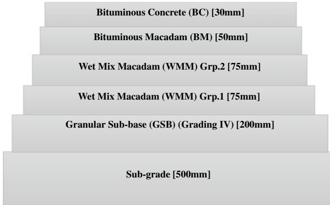
Fig. 2 Detailed design of flexible pavement
