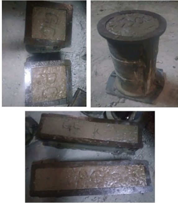
Fig. 1 GPC specimens after casting
