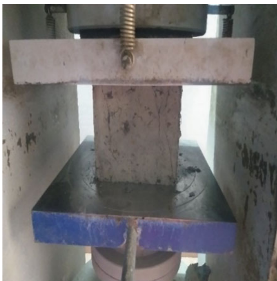
Fig. 4 Compressive strength test of cube
