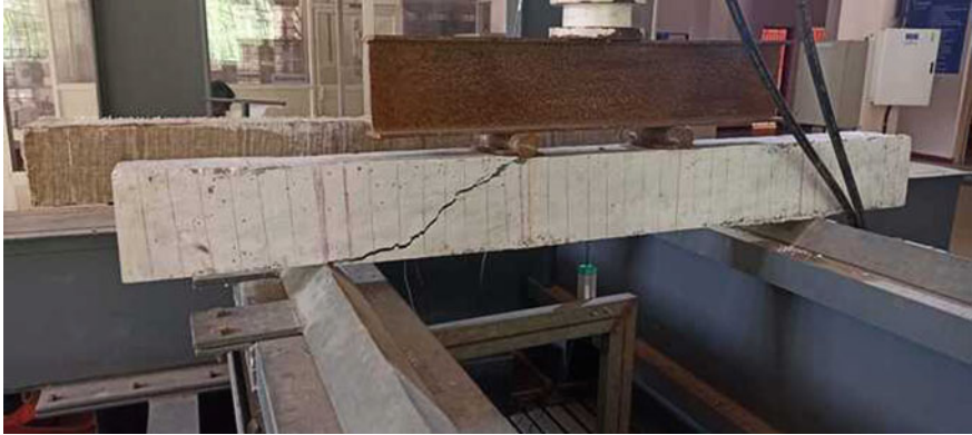
Fig. 8 Diagonal shear failure of un-strengthened beam
