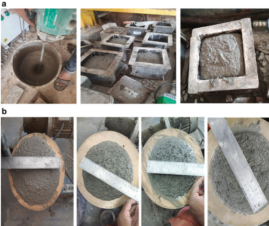
Fig. 2 a Casting of samples. b Flowability check on the mix with 0%,1%,1.5% and 2% glass fibre
