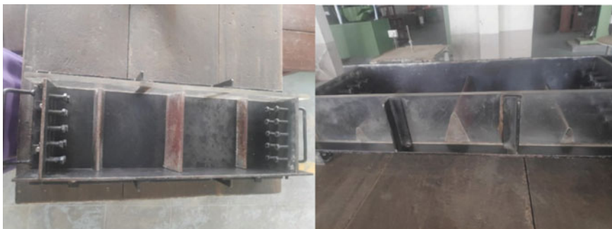
Fig. 1 Plastic shrinkage mould based on ASTM 1579
