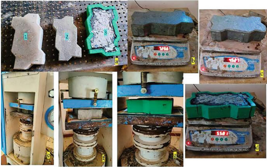
Fig. 7 a1 Factory made block, a2 block without frame, a3 block with frame, b weighing factory made block, c weighing block without frame, d weighing block with frame, e factory made block in CTM, f block without frame in CTM, g block with frame in CTM
