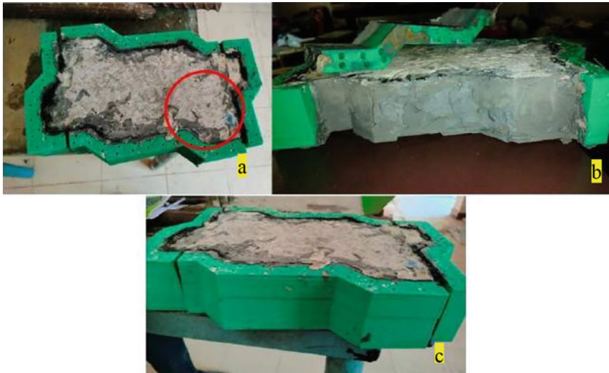
Fig. 8 a The only visible crack is on the surface, b no vertical crack in the sides, c block after loading in CTM
