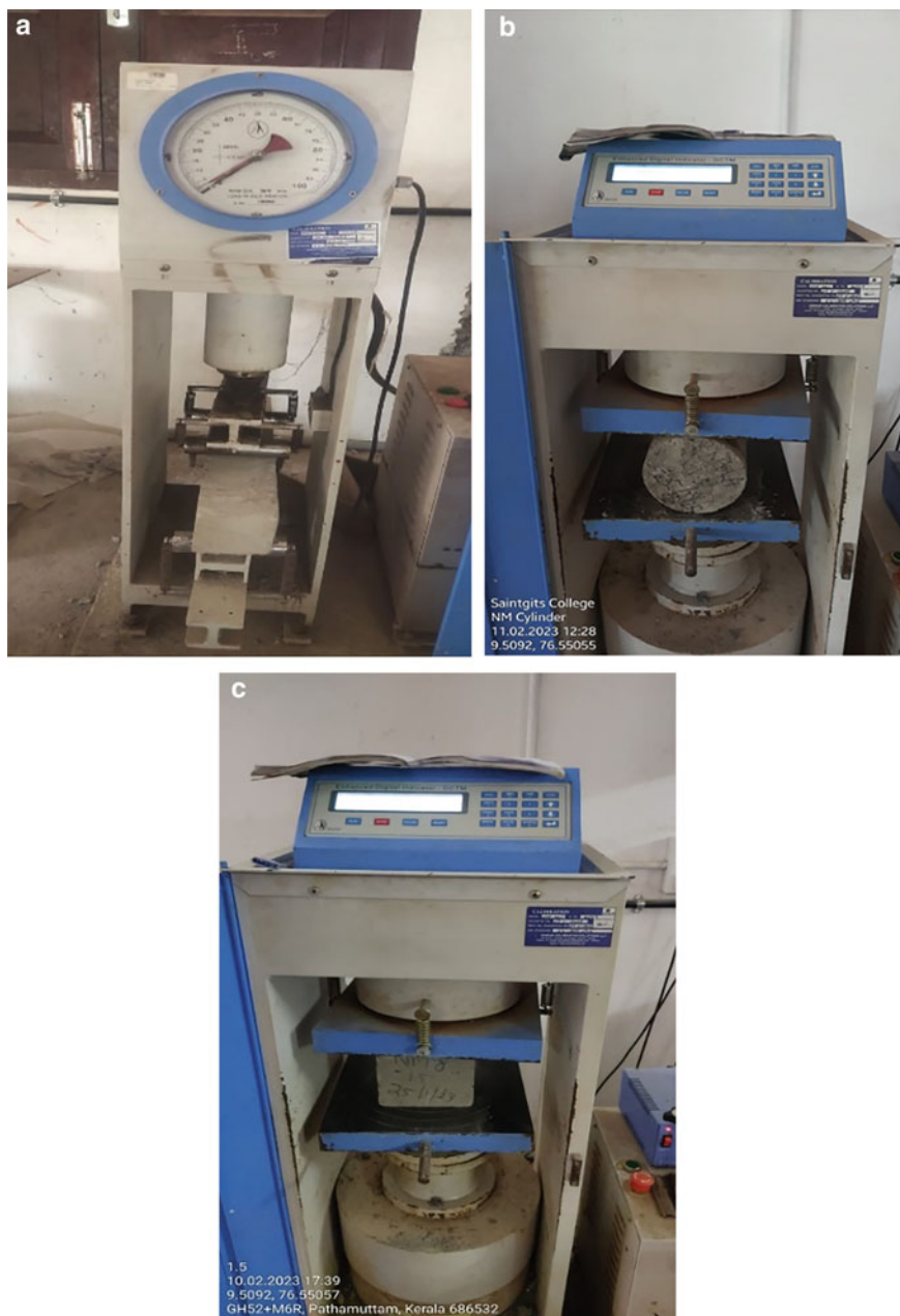
Fig. 1 a Test setup for flexural strength test. b Test setup for resistance measurement of split tensile test. c Test setup for resistance measurement of compressive strength
