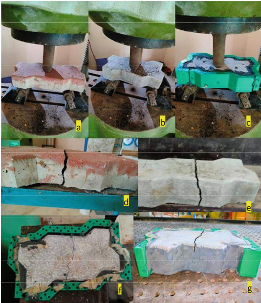
Fig. 10 a–c Three-point test setup of factory-made block, paver block with and without PETG frame, d–g crack pattern of factory-made block, paver block with and without PETG frame
