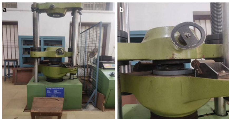
Fig. 3 a Experimental setup for compression testing, b CSTP specimen loaded in the compression machine
