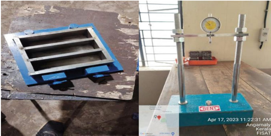
Fig. 1 Drying shrinkage mould and length comparator. When L_1 > L_2 ; Shrinkage = \frac{(L_1 - L_2)}{L_1} \times 100\% [5]
