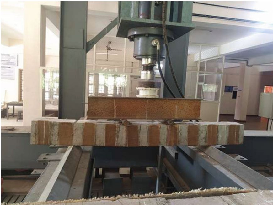
Fig. 10 Failure of partially wrapped beam
