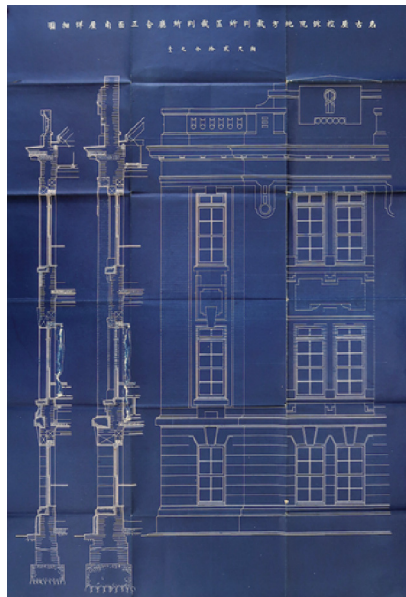
Fig. 4. A detailed cross-sectional drawing of the Nagoya Court of Appeal building
