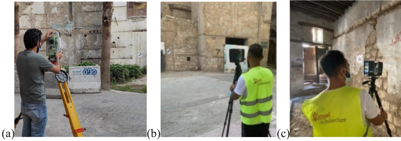
Fig. 8. (a) georeferencing the targets (b) canning the building's facades (c) Scanning the building from inside
