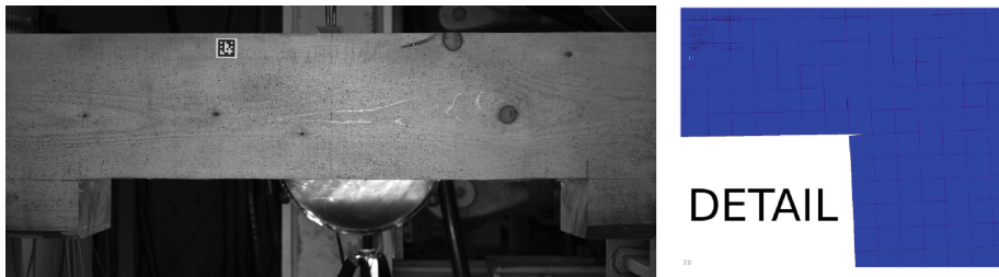
Fig. 5. The region of interest (left) in cracked mode after the experiment with cracks evident on both sides of the notch. The same domain (right) as detail of the numerical model (zoom in) also in cracked mode.
