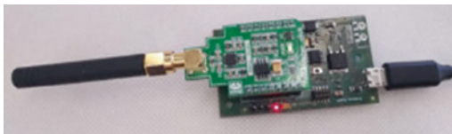
Fig. 20 Arancino Mignon end-node equipped with RF Meter sensor
