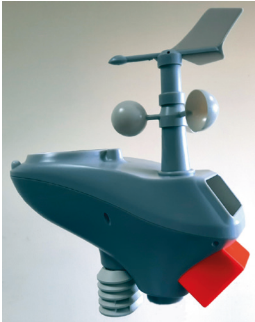
Fig. 14 AIR Environmental Station (SME-ES-02)
