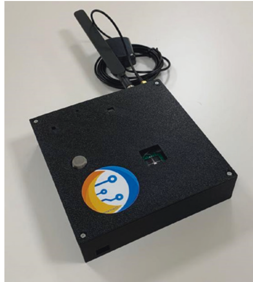
Fig. 15 Mobile Environmental Station (SME-ES-03)
