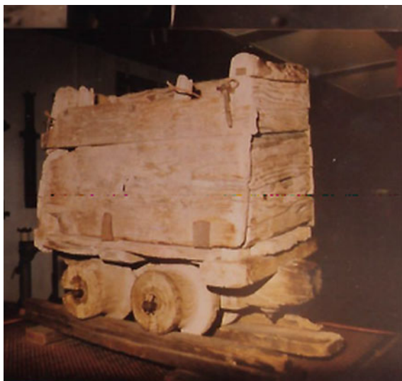
Fig. 3 Wooden mine car used to transport ores in the mines of the Apuseni Mountains (courtesy of Dr. V. Wollmann)
