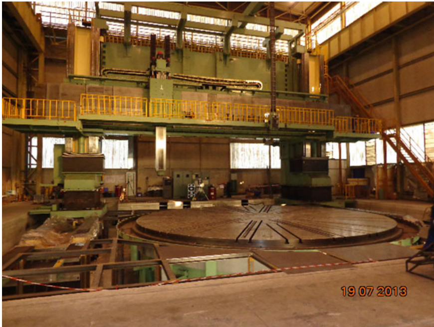
Fig. 12 Europe's largest carousel lathe, produced at ONSAL Roman (Photo from the author's collection)
