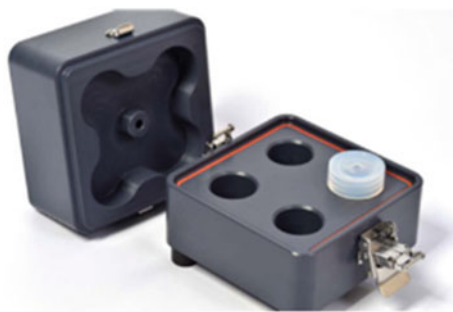
Fig. 3 The Mixed Odor Delivery Device (MODD) used to contain separated components within the device and release a mixed odor at the sniffing outlet, published by DeGreeff et al., Forensic Chemistry , vol. 4, 2017; licensed by Elsevier and Copyright Clearance Center (DeGreeff et al. 2017)
