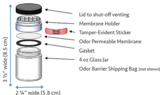
Fig. 1 SciK9 Training Aid Delivery Device (TADD) diagram, published by Sharpes et al., “Evaluation of the SciK9 Training Aid Delivery Device for Containment of Powders”, U.S. Army Combat Capabilities Development Command Chemical Biological Center, DEVCOM CBC-TR-1705; this document is in the public domain (Mach et al. 2021)
