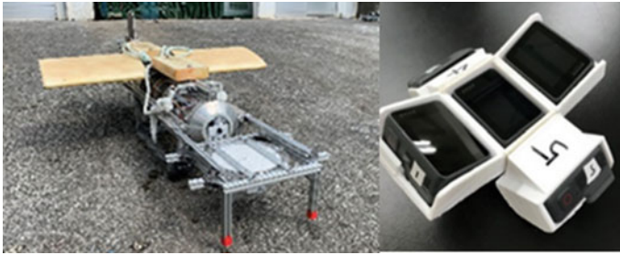
Fig. 6.1 Towed ROV with a multi-camera unit
