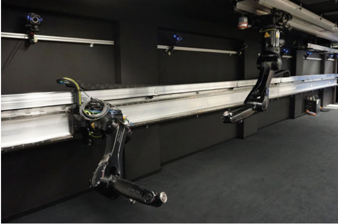
Fig. 3.7 The GRALS testbed, showing the 2 KUKA robots on their respective linear tracks and several of the VICON tracking cameras (copyright ESA)
