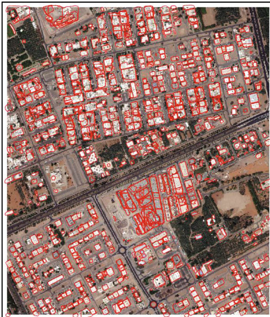
Fig. 9 AI building extraction for Al Ain project. Source: iSpatial Techno Solutions. (n.d.-d). Published with the company's permission
