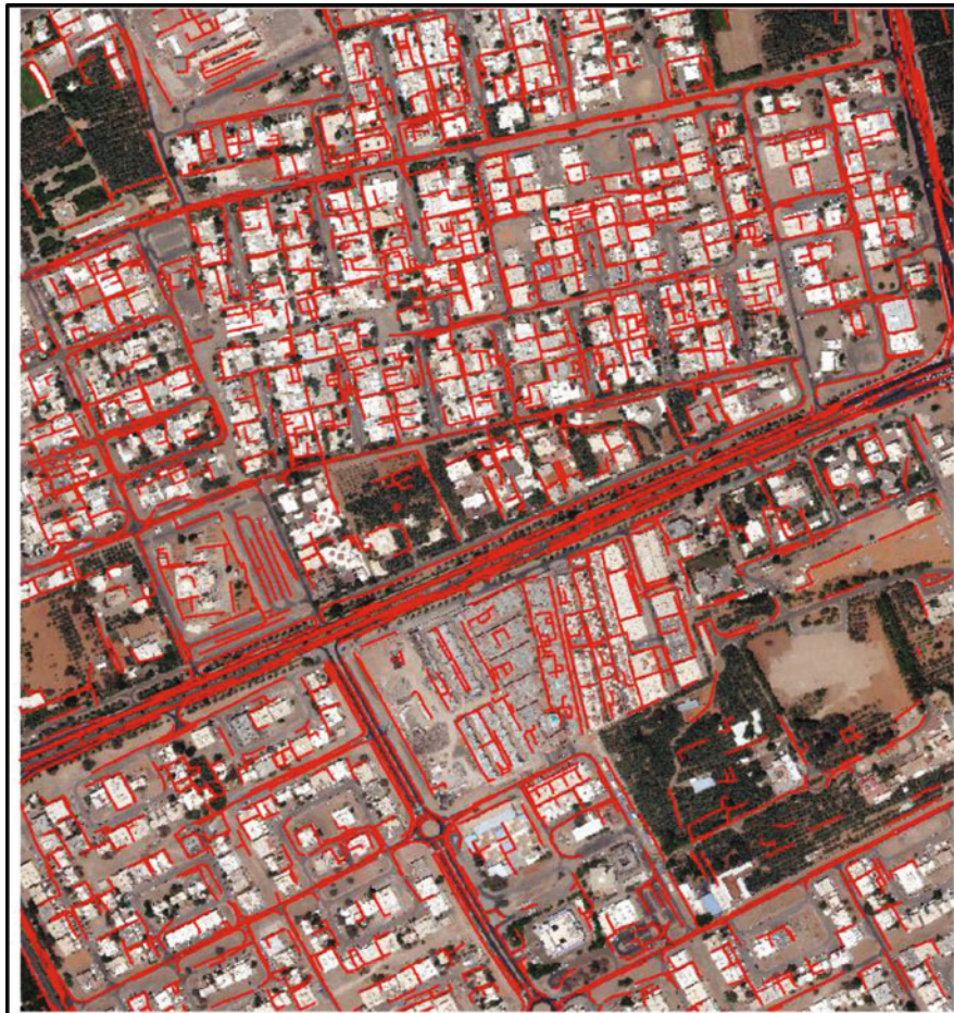
Fig. 11 AI road extraction for Al Ain project. Source: iSpatial Techno Solutions (n.d.-d). Published with the company's permission
