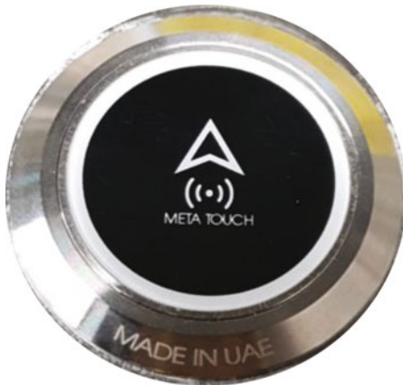
Fig. 7 The latest version of MetaTouch, TecK-v3.1. TecK-v3.1 is designed to be a master button, i.e., it can replace any elevator button. TecK-v3.1 is designed to function as a hybrid button, supporting both touchless (using radio-based distance sensor) and touch technology (built-in button). Source: MetaTouch. Published with the company’s permission
