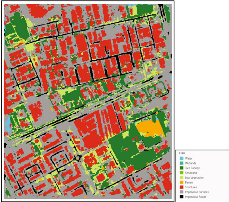
Fig. 12 AI image segmentation for AI Ain project. Source: iSpatial Techno Solutions. (n.d.-d). Published with the company's permission
