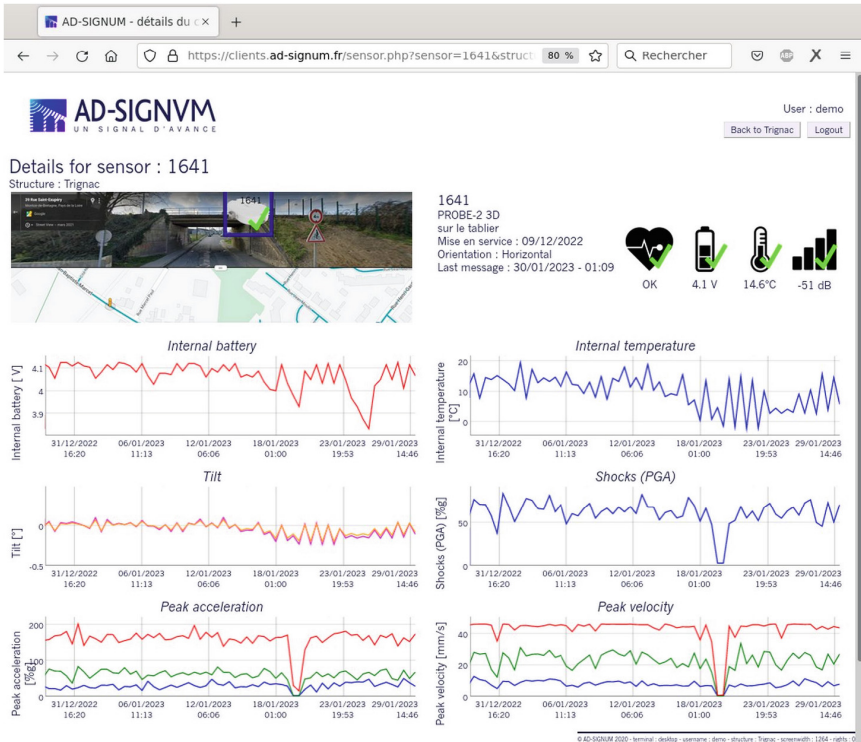
Fig. 7. Main page for the PROBE-2 sensor installed on Trignac PRA. Showing detailed SOH over the period 2022/12/30 – 2023/01/30.
