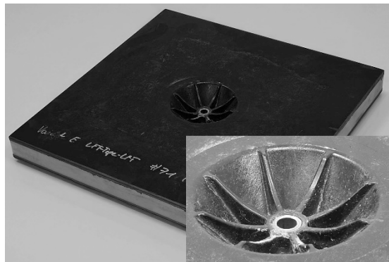
Fig. 11.2 Breadboard sandwich specimen with central load point and LFT load point support structure for validation on structural level.
