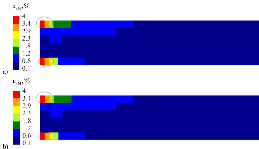
Fig. 2.11: Distributions of von Mises equivalent strain in a beam area. a) - direct solution of 7 creep and plastic problems; b) – calculations with use of Eq. (2.24).
