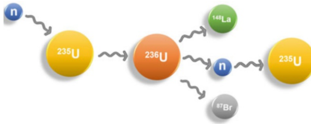
Fig. 4.2 A neutron (blue) colliding with 235 U (yellow) and inducing a fission event in which the 235 U nucleus splits into smaller components: 148 La, 87 Br, and an
