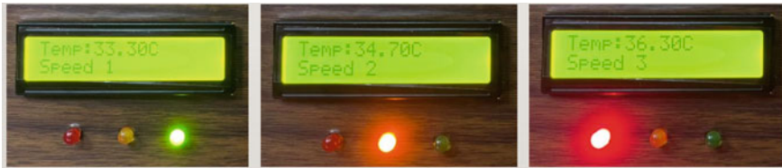
Fig. 3.6 LCD display when detected changing of temperature and speed of fan
