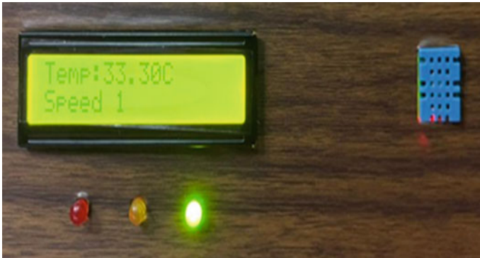
Fig. 3.5 Speed and LED monitoring system
