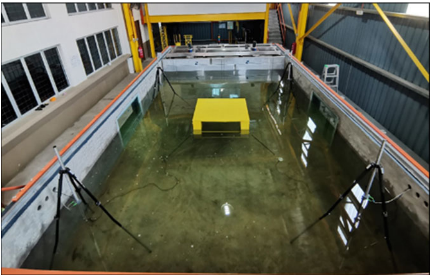
Fig. 16.4 Semi-submersible platform in the wave tank during the experiment
