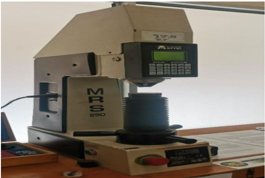
Fig. 13.2 Universal hardness test
