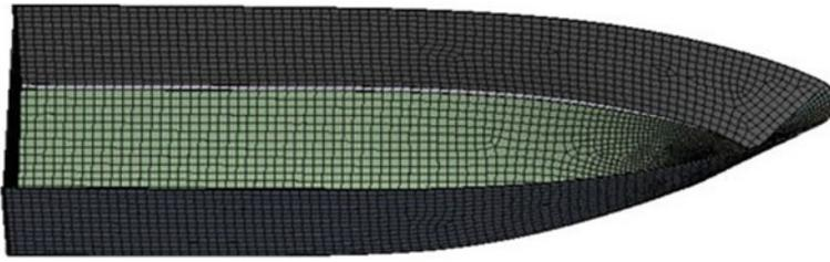
**Fig. 12.5** The completed mesh of the hull
