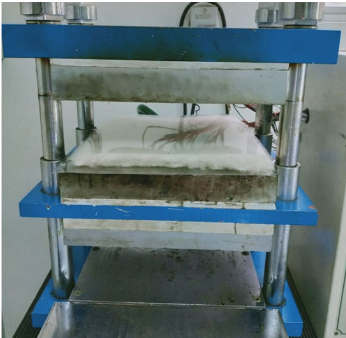
Fig. 23.2 Hydraulic hot-pressing of web kapok into nonwoven mat with higher strength
