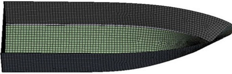
Fig. 12.5 The completed mesh of the hull
