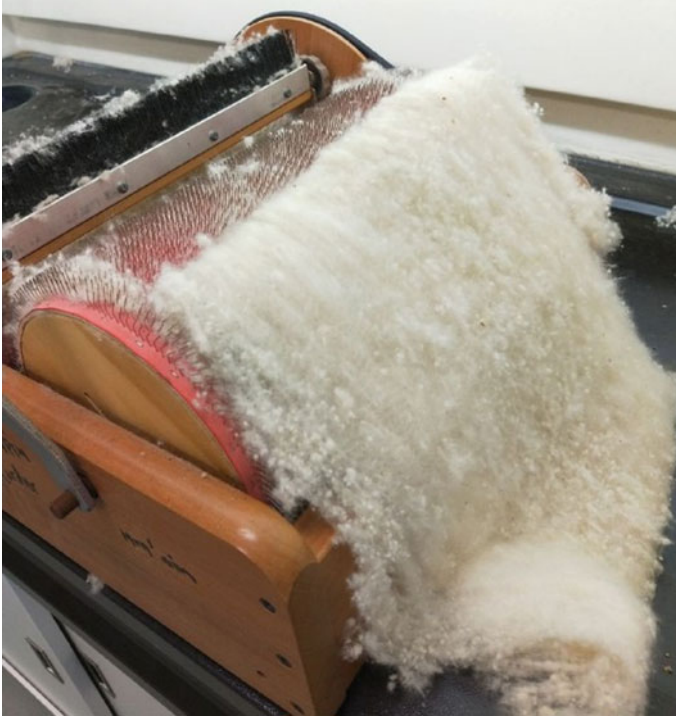
Fig. 23.1 Kapok fiber web produced using Ashford drum carder
