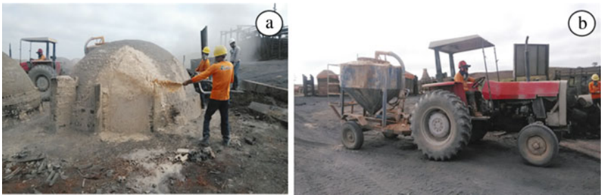
Fig. 3 Cooling of the kilns through the application of water and clay (a) with the aid of a tractor, Massey Ferguson 275 model (b) (Source The authors 2023)
