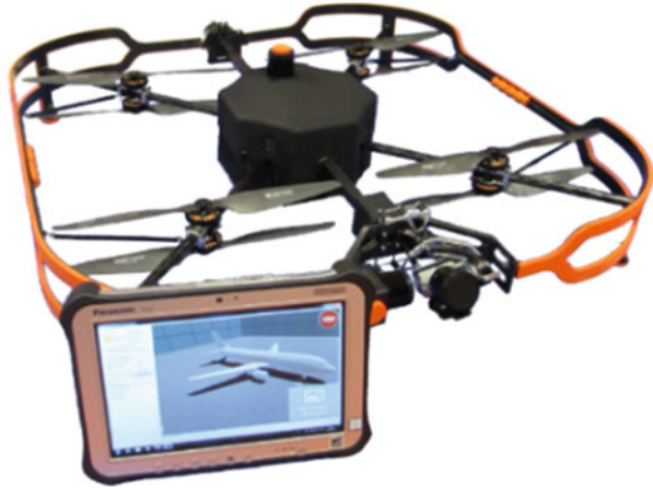
Fig. 1 Drone for aircraft maintenance inspection. (Source: airbus.com )
