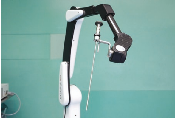
Fig. 4.1 The three electromagnetic locks of the ENDOFIXexo allow any position to be taken within arm range. Reference: Hintschich, C. A., Fischer, R., Seebauer, C., Schebesch, K.-M., Bohr, C. & Kühnel, T. (2021). A third hand to the surgeon: the use of an endoscope holding arm in endo-nasal sinus surgery and well beyond. European Archives of Oto-Rhino-Laryngology , 279(4), 1891–1898. https://doi.org/10.1007/s00405-021-06935-x
