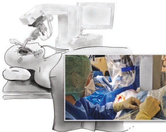
Fig. 9.5 Schematic drawing of the robotic ENT system RobOtol® of the company Collin using a CI electrode array holder to position and advance the array into the cochlea. A conventional, open surgery is necessary before the robot can be used for this application because the system needs some space to rotate around its pivot point. The system can also be used to manipulate through the external ear canal
