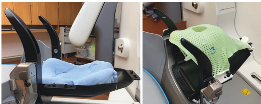
Fig. 8.2 Mask adapter for Gamma Knife Icon. Mendel J T, Schroeder S, Plitt A, et al. (March 19, 2021) Expanded Radiosurgery Capabilities Utilizing Gamma Knife Icon™. Cureus 13(3): e13998. doi:10.7759/cureus.13998
