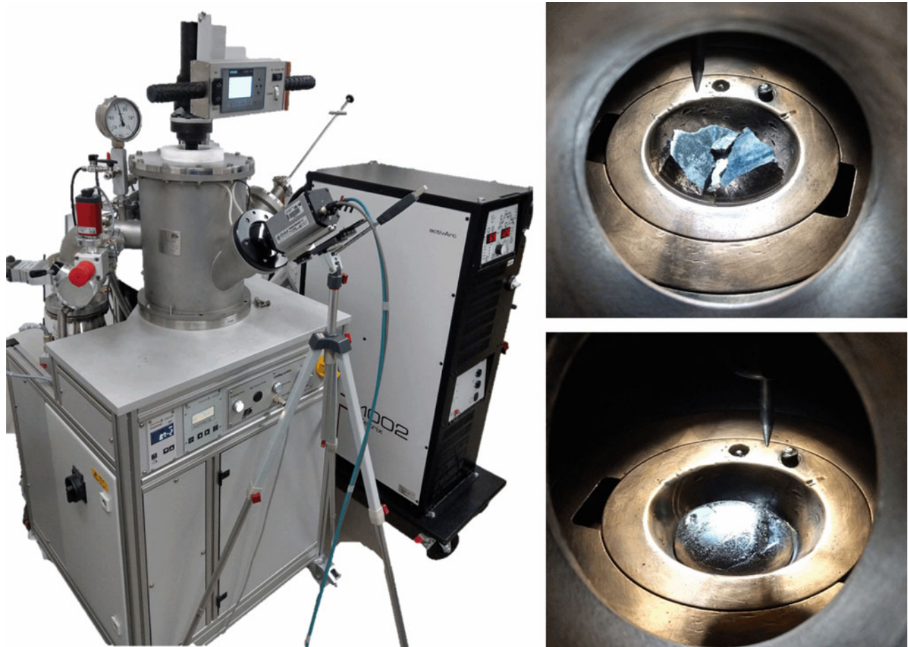
Fig. 3 Arc melter setup at Access technologies GmbH with thermal imager (left); Cu-mold with crushed material before trial (top right); Cu-mold with remolten material after trial (bottom right)
