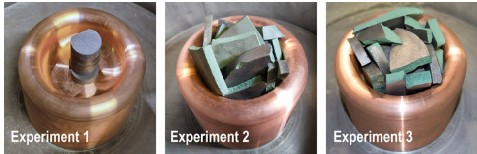
Fig. 2 Crucibles loaded with MnO raw material for each of the experiments. Experiments 1 and 2 used pure MnO, while experiment 3 used 15 wt.% iron and 85 wt.% MnO
