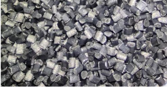
Fig. 3 10 wt% SCF reinforcement PA6 compounds
