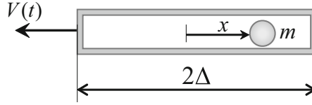
Fig. 1.12 Mass m , whose position inside the moving container is described by the relative coordinate x(t) , is subjected to a periodic stepwise loading and reaction impulses from the vertical walls as the container's velocity is varying according to the triangle wave law, V(t) = V_0\tau(\omega t)
