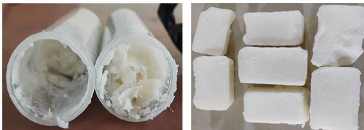
Fig. 2 (a) Initial preparation of soap base in Tarsons (b) Preparation of soap base cubes
