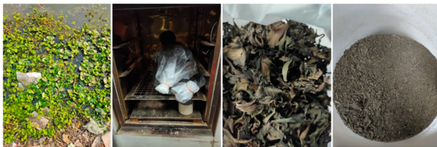
Fig. 4 Pond infested by water hyacinth, cleaned and washed sample, dried leaf sample, and acquired WHB (left to right)
