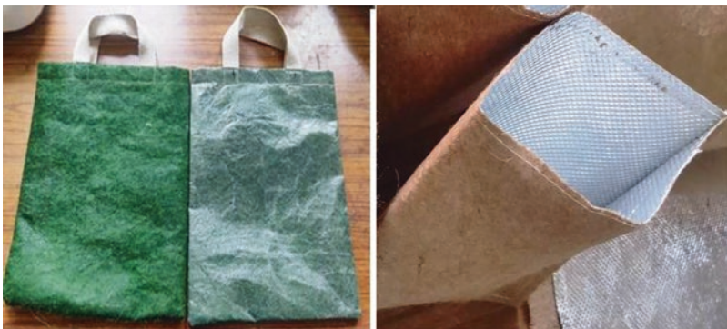
Fig. 8 Bag from laminated nonwoven (polyethylene and aluminum foil). (Report, 2021 [18])
