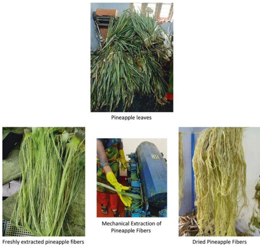
Fig. 8 Mechanical pineapple leaf extraction
