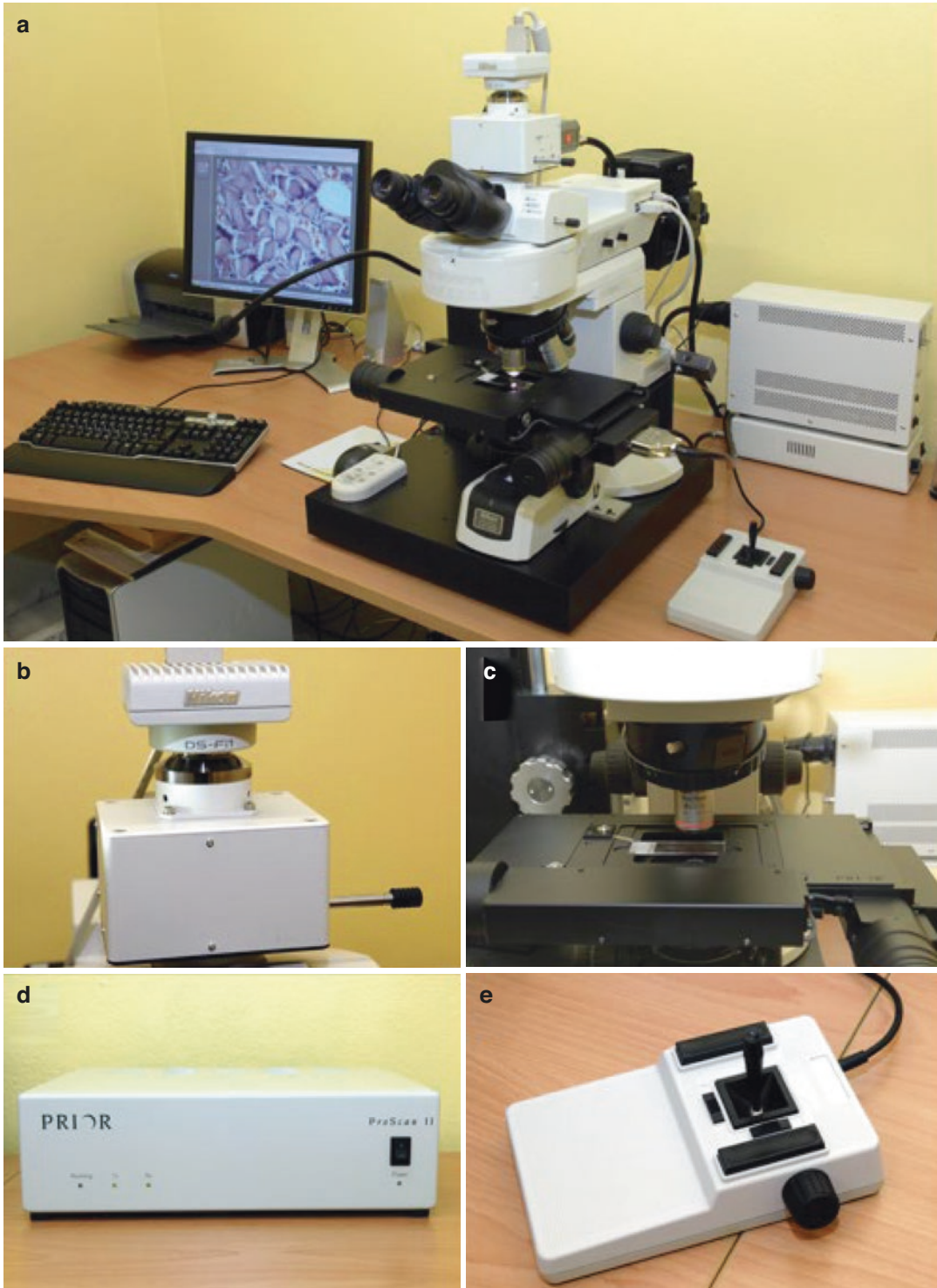
Fig. 17.7 (a) Shows an overview of a computer-based microscope system for histomorphometry, consisting of a light microscope (Eclipse 80i, Nikon, Japan) with a connected digital camera (Nikon DS-Fi1, Nikon, Japan) (b),
