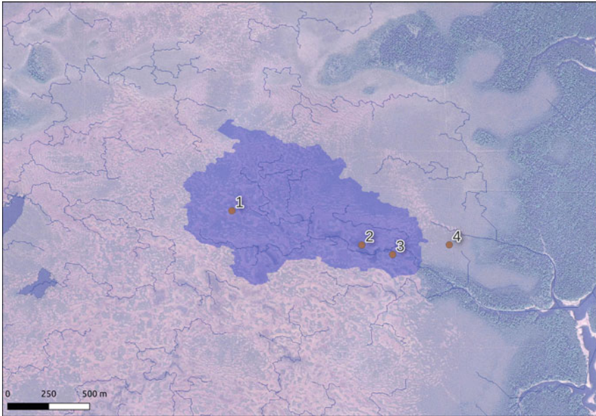
Fig. 14.1 Stream catchment area (blue shade) and piezometer location (1—hollow, 2—ridge-hollow ecotone, 3—pool, 4—ryam)
