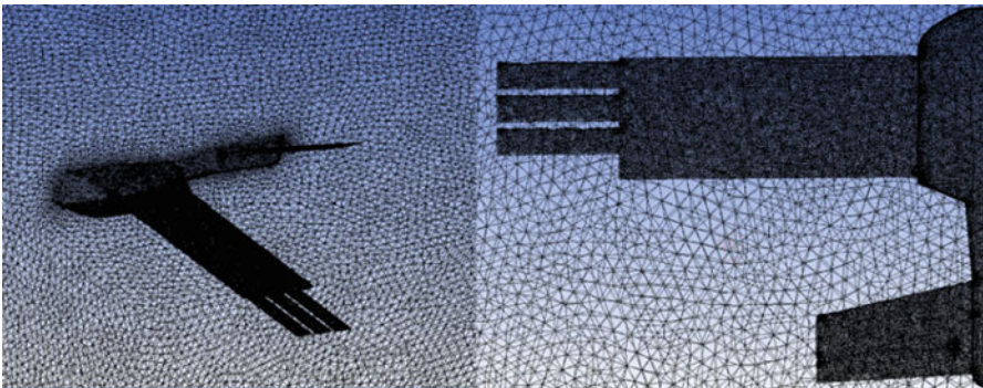
Fig. 2 Details of the unstructured mesh
