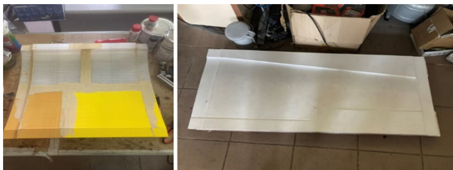
Fig. 3 3D printed mold (left). The MDF wood mold (right)
