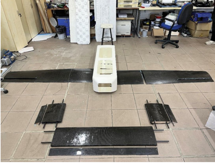
Fig. 6 The hybrid UAV in the assembly phase
