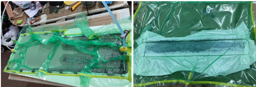
Fig. 4 Resin infusion process (left). Vacuum bagging process (right)
