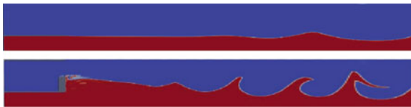
Fig. 2 Comparison between the mixing degrees when including a bluff body in two concentric jets. Volume fraction is plotted, and the two colors represent each one of the flow phases
