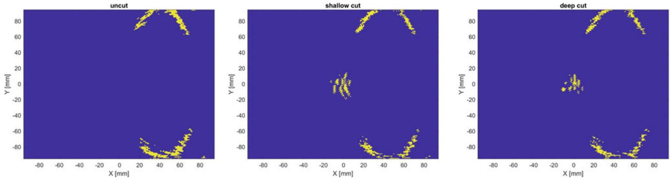
**Fig. 6.3** Results of clustering; clusters indicating: (a) edges reflection (reference measurement); (b) damage reflection and edges reflection (measurement for shallow cut); and (c) damage reflection and edges reflection (measurement for deep cut)
