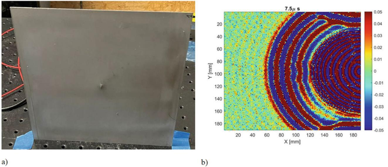
**Fig. 6.1** (a) View of the samples from the laser scanned side; (b) the registered guided wave propagation: Two wave modes are visible with different wavelengths
