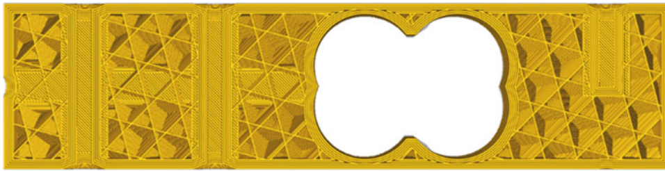
Fig. 18.2 Filament pattern of the additive manufacturing load cell prototype
