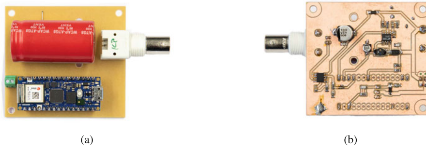
Fig. 8.4 Prototype hardware with the dominant capacitor where the energy for the impulse is stored. (a) Top. (b) Bottom
