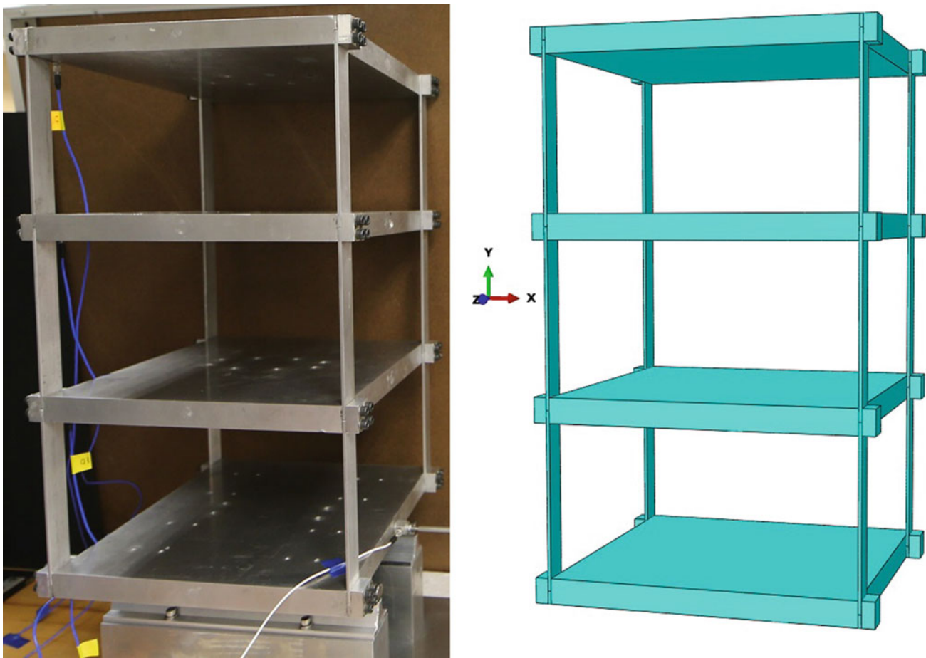
Fig. 12.5 The actual 4-story structure next to the geometry used in the ABAQUS models
