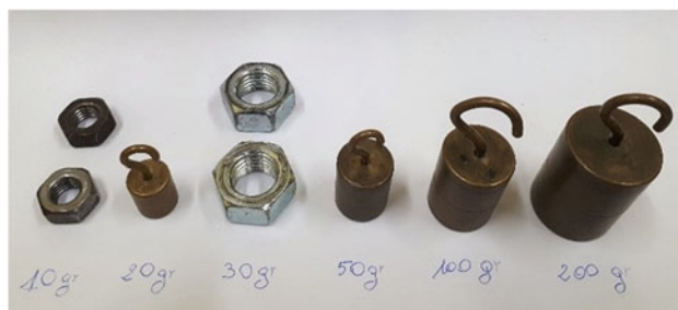
Fig. 19.9 Set of masses for the static loading conditions
