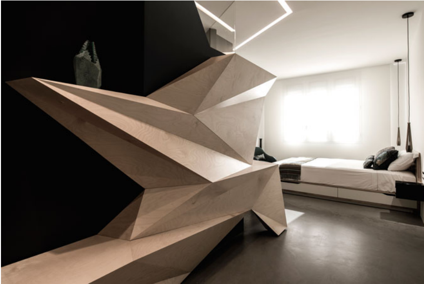
Fig. 2 Digital wood: the architectural furniture is made of self-supporting sub-modules. All facets are designed through a computational procedure that generates all geometrical features necessary for the six-axis circular-saw robotic-cut carried out directly at ALO laboratory
