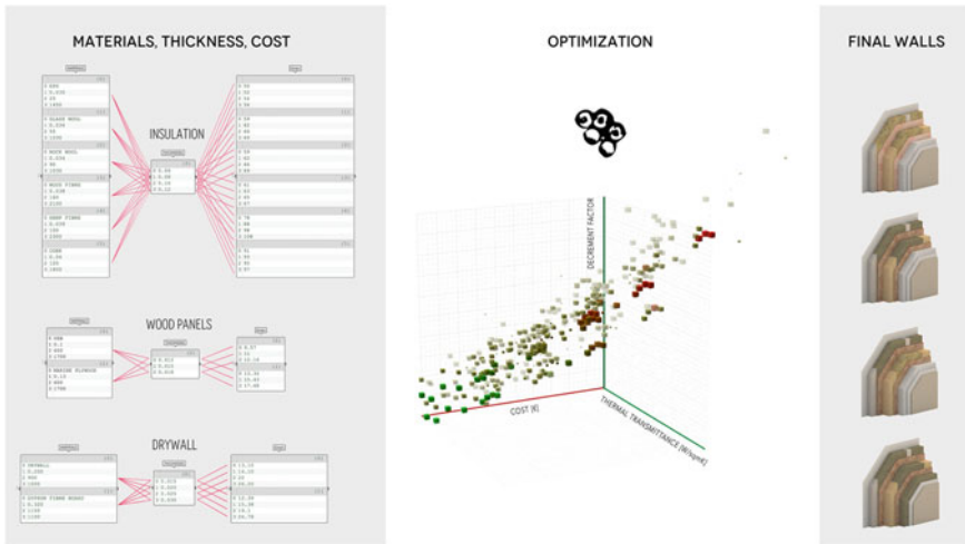
Fig. 4 The optimization process through Octopus for Grasshopper combines materials and thicknesses while maximizing time shift and minimizing thermal transmittance, decrement factor and costs
