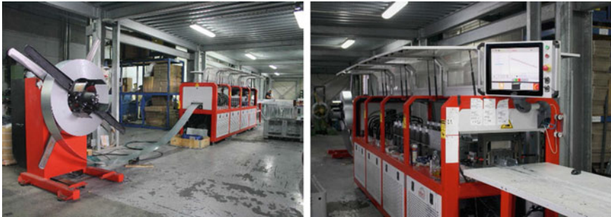
Fig. 13 Arkitech AF I 200P framer. Manufacturing process file to factory
