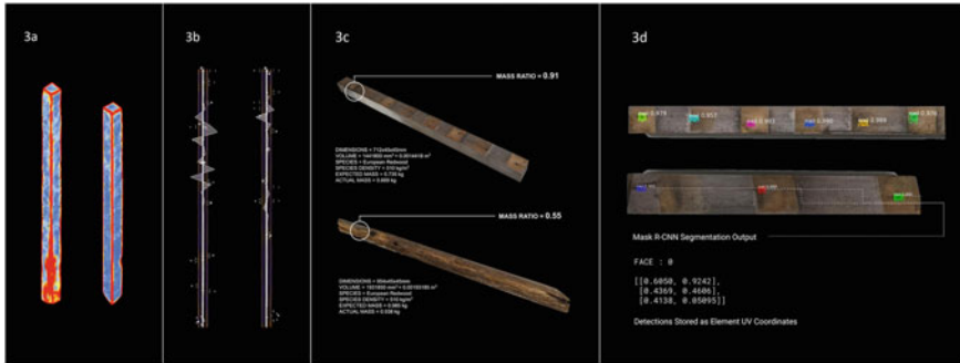
Fig. 3 a Surface curvature analysis. b Two examples of mesh curvature visualization. c Example mass ratios for structurally usable vs a highly decayed wooden element. d Example output when localizing texture defects using Mask RCNN
