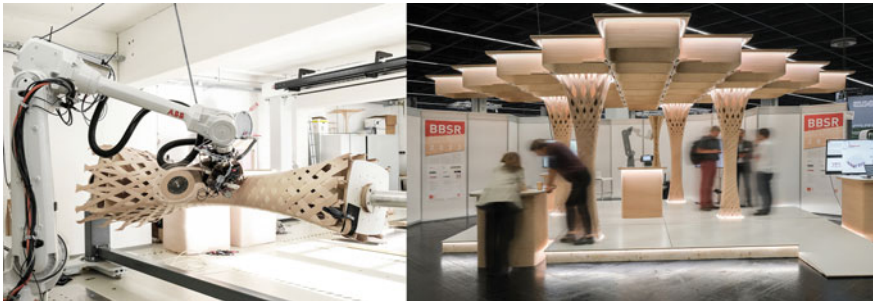
Fig. 9 The 3DWoodWind project uses strips of thin veneers to and industrial robots to wind structural components as columns and modular ceiling components for full-scale architectural structures. Right: The BBSR Research Prototype was presented at the Digitalbau 2022 in Cologne
