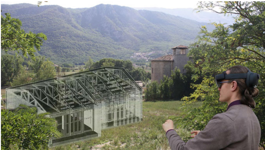
Fig. 10 HoloLens 2 used to visualize the dwelling in the lot (immersive AR)
