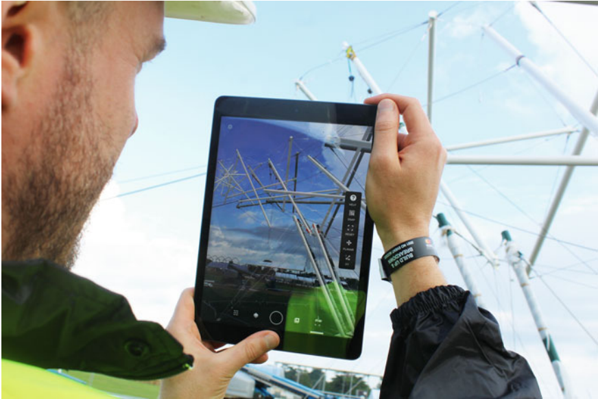
Fig. 7 Comparing the Real and Calculated Position in AR
