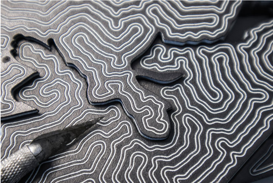
Fig. 10 Detail of the conductive graphite pattern of the touch feelers prototype
