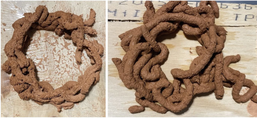
Fig. 1 Left: first trial—manual extrusion. Experiment: Clay 85% and Hemp 15%. Right: second trial—manual extrusion. Experiment Clay 85% and Hemp 15%
