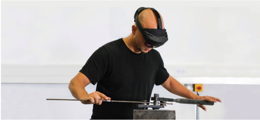
Fig. 10 Three-dimensional rebar bending in MR
