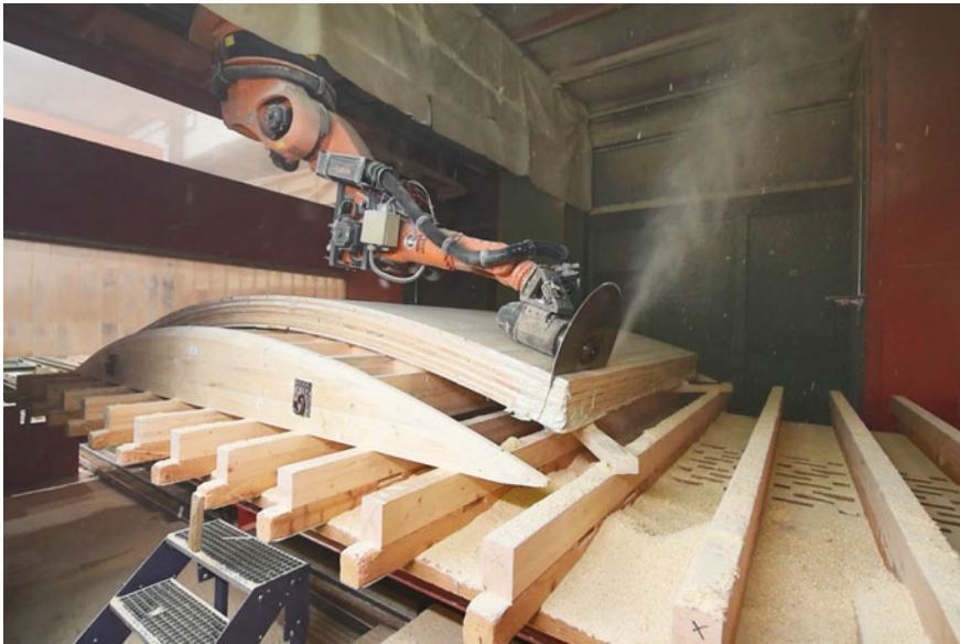
Fig. 1 Large-scale robotic fabrication process defined in a visual programming environment at ZÜBLIN Timber, Germany
