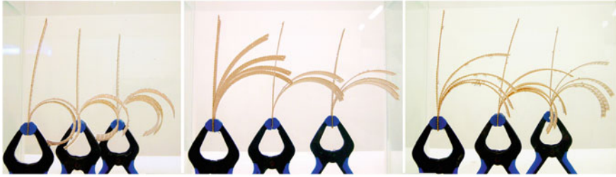
Fig. 6 Different curvatures and velocity of curvature of similar 3D printed specimens with different printing properties
