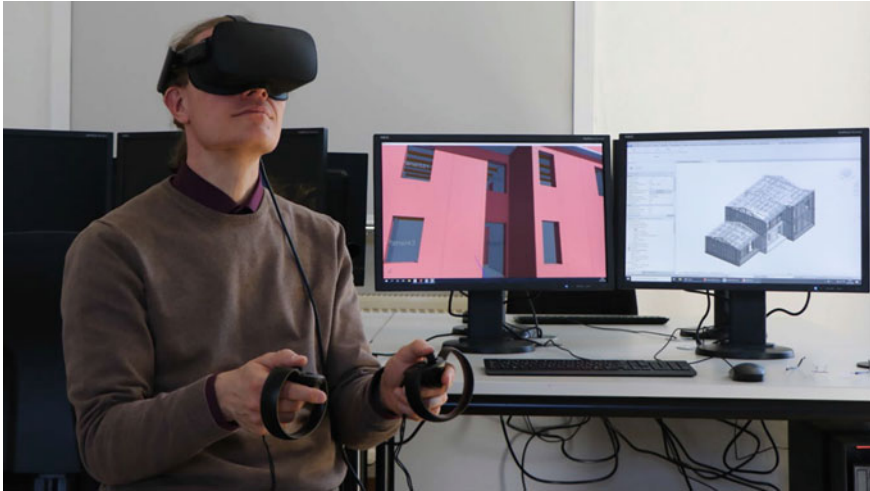
Fig. 8 Oculus rift (immersive VR). One person has a VR vision and people can see the 3D model on the screen
