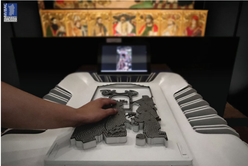
Fig. 8 The figure shows the APTICA interfaces with the 3D miniature of the artwork. The dark top surfaces are the touch feelers, sensing surfaces that enable the multimedia contents navigation
