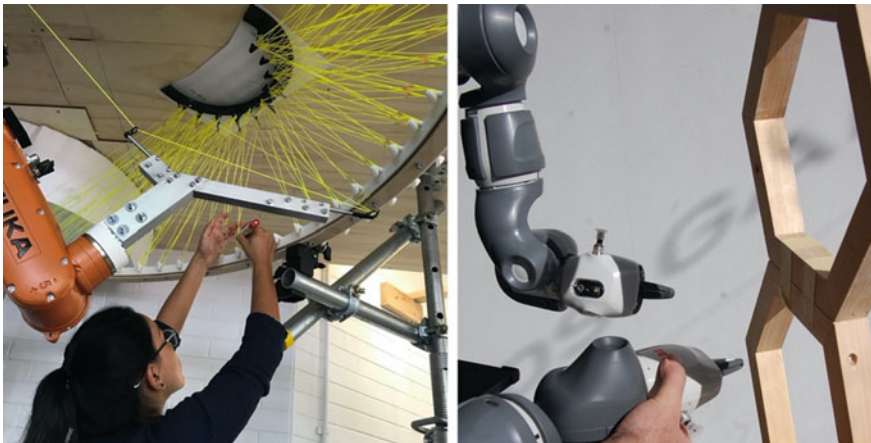
Fig. 5 Cooperation to Collaboration: human support of robotic fabrication process for robotic carbon fibre winding (Reinhardt et al, 2017, left), versus data capture for fabrication techniques and knowledge of motion, force and material resistance (Reinhardt et al, 2016, right).
