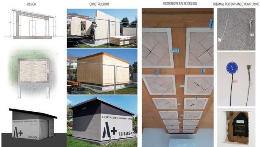
Fig. 7 The test room has been designed and built to experiment in reality what had been digitally simulated, concerning in particular the responsive false ceiling and the optimized timber walls
