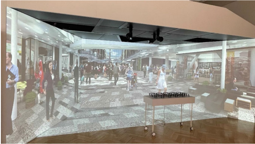
Fig. 6 Cave automatic virtual environment and associated 3D glasses applied for the open debate between designers, enterprises and members of department of civil protection to improve the winning project (VR space)
