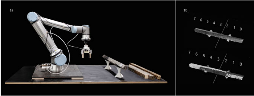
Fig. 1 a The UR10 in combination with the gripper-scanner tool and the scanning holder. b For the scanning process, each side requires seven camera captures to be registered afterward
