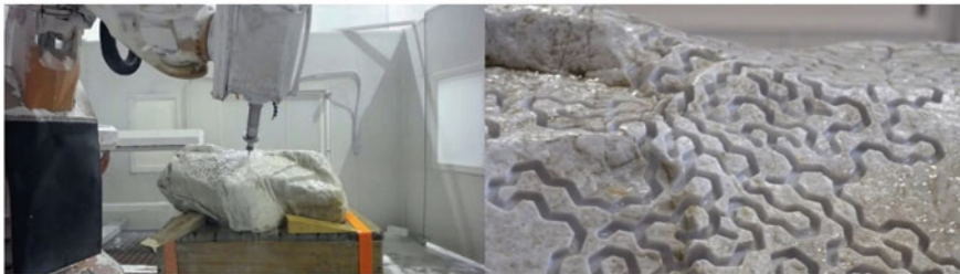
Fig. 11 Left—Fabrication using 7 axis milling, Right—Milling details
