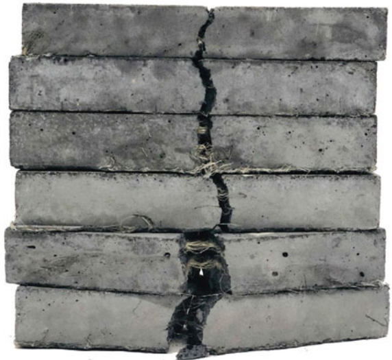
Fig. 14 Comparison of the flexural strength of BCMs and BGCs of specimens with and without hemp fibre
