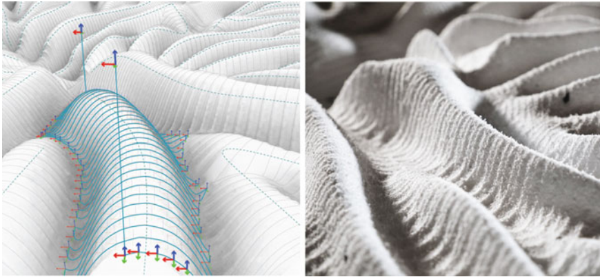
Fig. 9 Left: Robotic toolpath for the contouring perpendicular to structural ribs of RD Slab 02 and mesh visualisation of the milled EPS formwork; Right: Image of a milled EPS formwork
