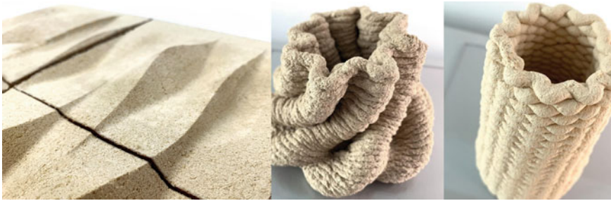
Fig. 12 Left: Compacted and milled acoustic elements from used wood particles and starch. Right: Investigations in a 3D-printable, 100% bio-based wood paste
