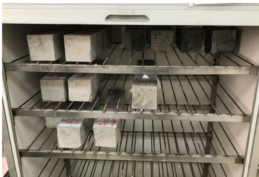
Fig. 3 Holding concrete samples in a normal hardening chamber
