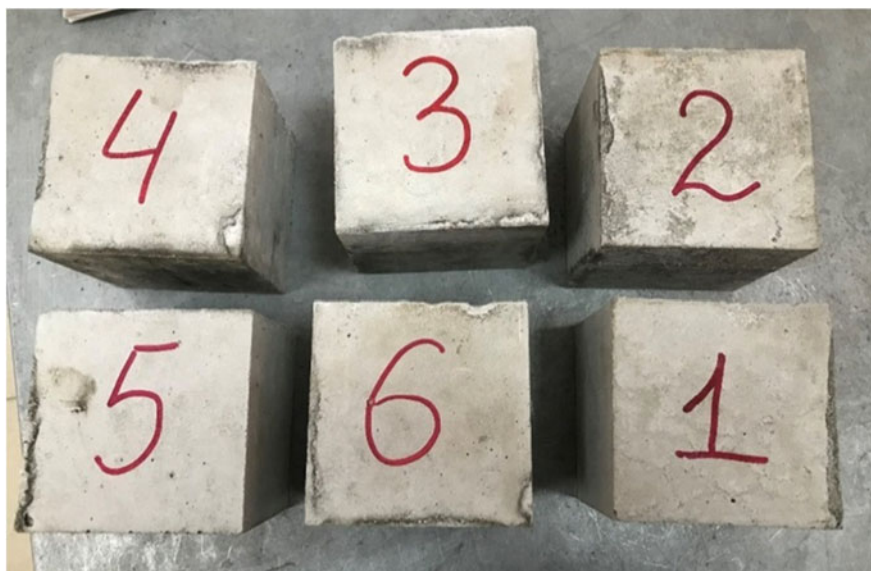
Fig. 1 Manufactured samples-concrete cubes
