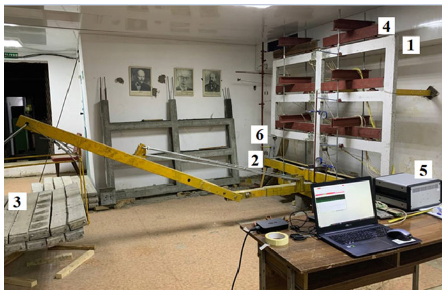
Fig. 1 Test installation: 1—Prototype, 2—lever-suspension system, 3—design load, 4—distribution beams and strands, 5—strain gauge station, 6—collapsible mechanism
