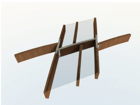
Fig. 7 A fragment of a grid of a timber closed circle-mesh vault on a square plan
