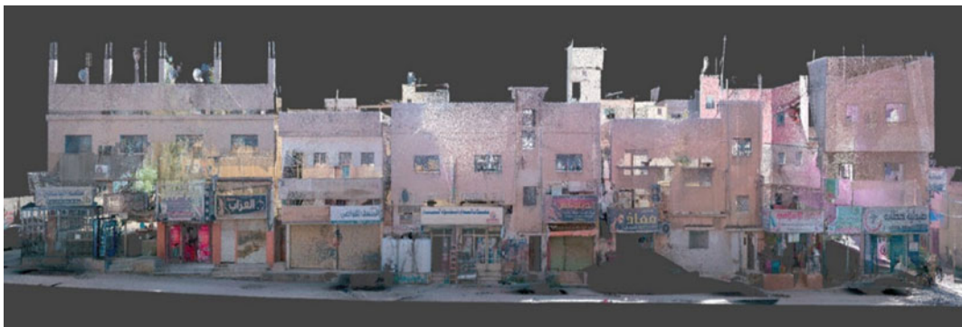
Fig. 28.8 Screenshot of the point cloud showing an urban front after applying the noise reduction filter
