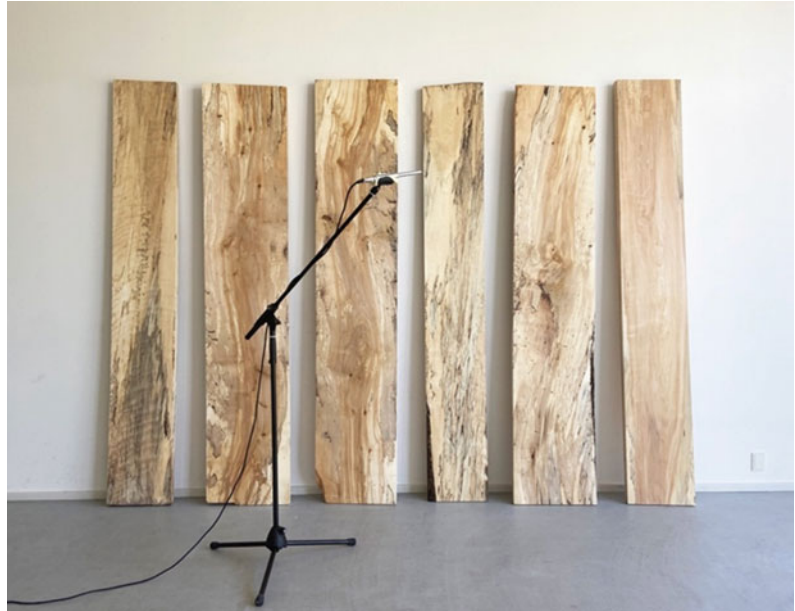
Fig. 10 Room acoustic measurements with free standing poplar planks
