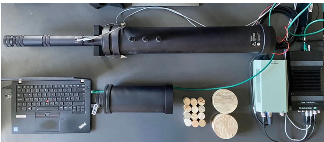
Fig. 4 Impedance Tubes testing instrument used for material acoustic analysis, including both large wide tube (low frequency analysis), small tube (middle and high frequency analysis), signal generator and specific computer/software for analysis, post-processing and export of results
