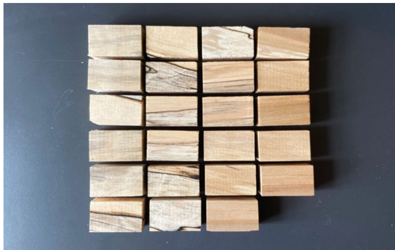
Fig. 3 Set of material samples that are examined for density variance, with lowest density in top left corner and highest density in lower right corner
