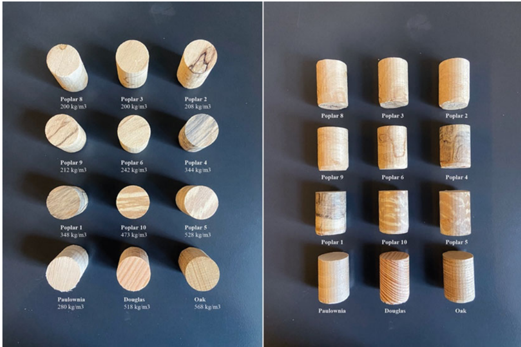
Fig. 5 Material samples (29 mm) prepared for Impedance Tube testing, including Poplar, Paulownia, Oak and Douglas fir wood species
