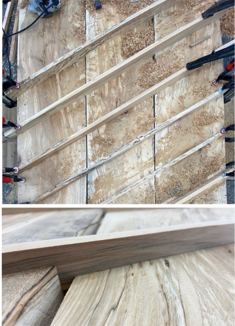
Fig. 9 Second full-scale cross-layer prototype with 60-degree crossing over three planks
