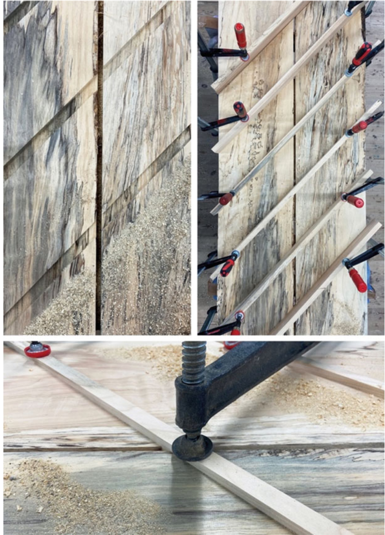
Fig. 8 First full-scale cross-layer prototype with 45-degree crossing over two planks
