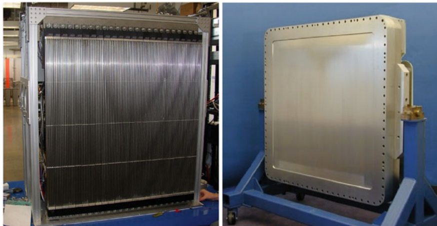
Fig. 3.37 Two methods of achieving 2D, or areal , detector coverage. ( left ) A vertical arrangement of individual 1D LPSDs (Reuter–Stokes). ( right ) A detector constructed with true 2D readout (ORDELA, Inc.)
