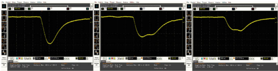
Fig. 3.13 Oscilloscope traces of typical neutron pulses from a ^3\text{He} proportional tube. The vertical scale is 100 mV per division and the horizontal scale is 200 ns per division for all
