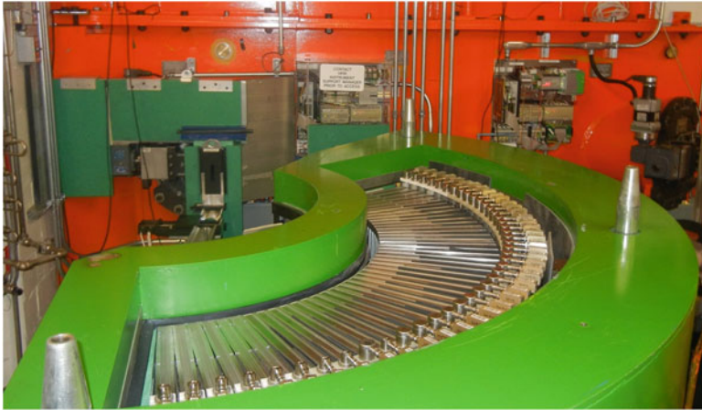
Fig. 3.36 Forty-four single-output tubes comprising a curved 1D detector array. (HB-2A Powder Diffractometer, HFIR)
