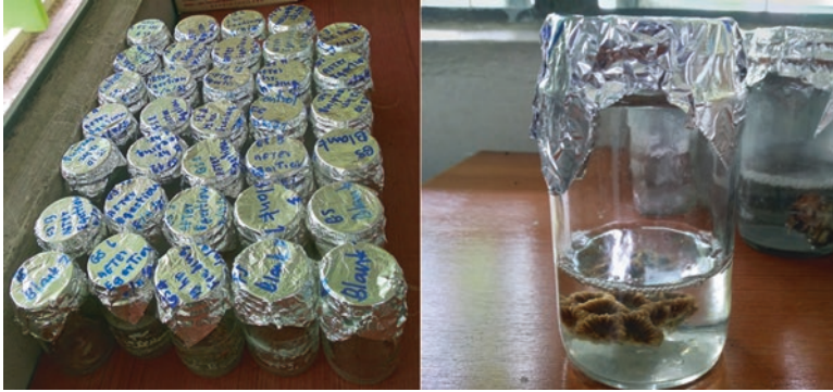
Fig. 7 Corals soaked in 3% formic acid for decalcification for seven days to soften the polyps and dissect it for extracting retained microplastics
