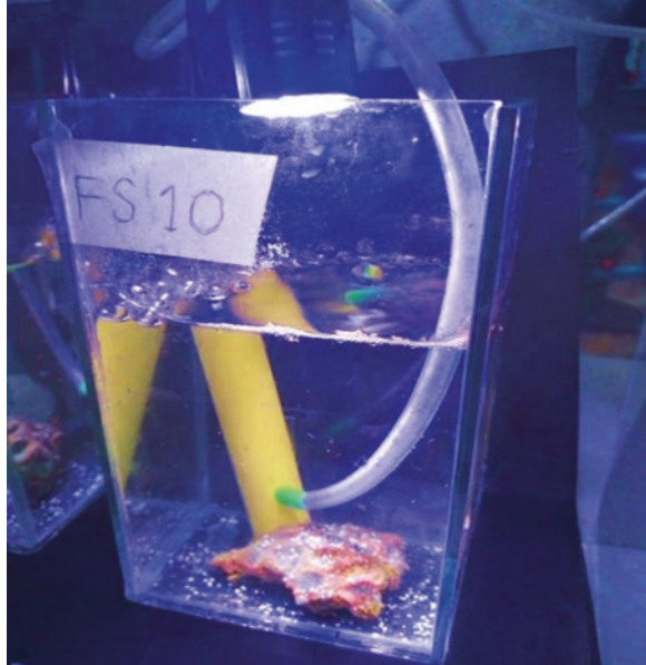
Fig. 4 Ingestion chamber with inlet flow to keep microplastics in flow and within the reach of corals. This picture shows Dipsastraea speciosa in ingestion chamber
