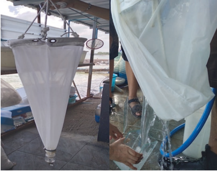
Fig. 2 Phytoplankton net of mesh size 60 \mu\text{m} was used to filter seawater, to screen any zooplankton, phytoplankton, or micro-particles present in the seawater used for acclimatization. This was done to ensure no other food particles are available for corals apart from the one provided during experiment. This filtered seawater was then used to wash, rinse and fill tanks for the experiment
