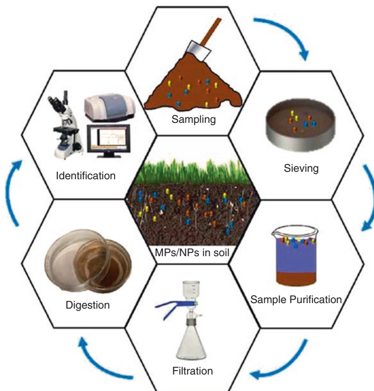
Fig. 2 Extraction of microplastics from soil. (Reproduced with permission (Junhao et al. 2021), copyright Elsevier, 2021). MP microplastic, NP nanoplastic
