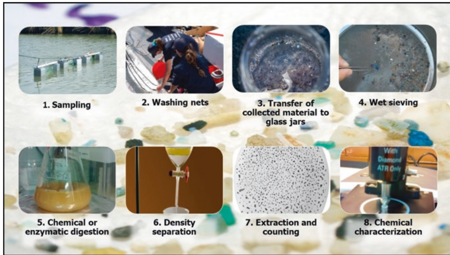
Fig. 5 Sampling and extraction of microplastics from water. (Reproduces from (Campanale et al. 2020). Copyright MDPI, 2022)
