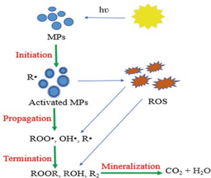
Fig. 4 Mechanism of microplastic degradation by photolysis. MPs microplastics, ROS reactive oxygen species
