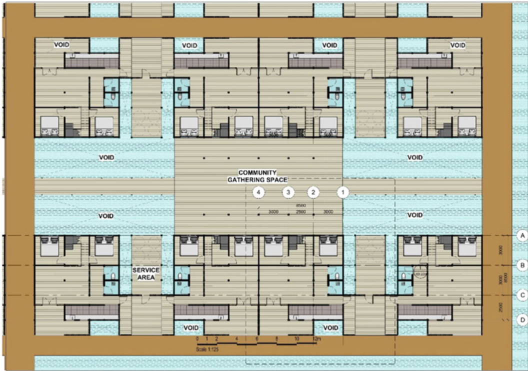
Fig. 4.12 Cluster planning at platform level with public and private amenities to support homestay programs in new water village planning model (Illustration by: Nor Efenday)
