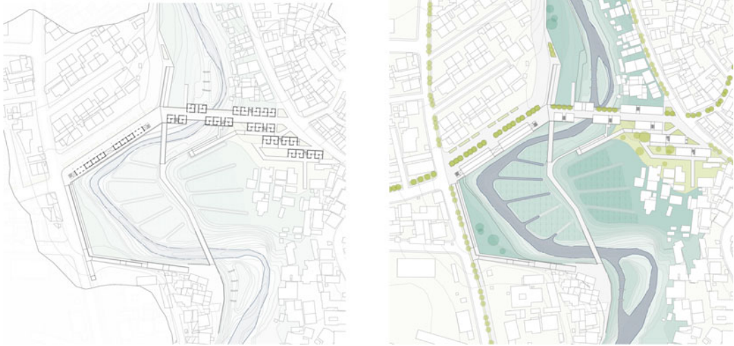
Fig. 3.4 General ground plan and flooding plan. Ground plan (left): the floor plan of housing and marketplace along with the river during normal conditions. Flooding
