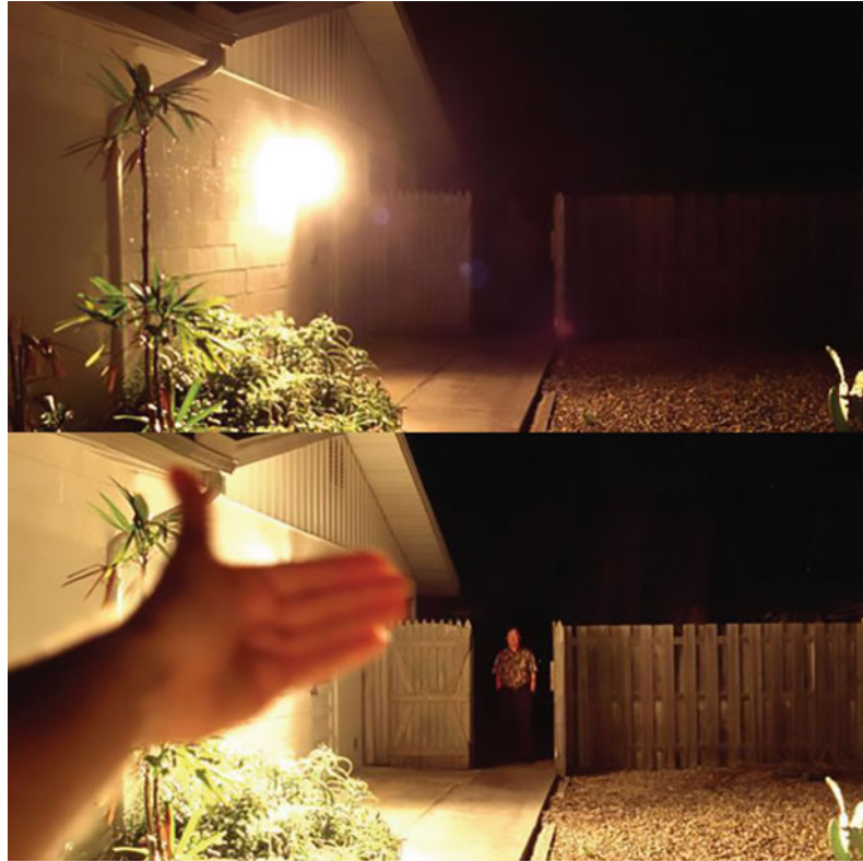
Fig. 26.5 Illustration of how glare limits the vision and how shielding the light improves visibility. Notice the discernability of the man in the gate and how the shadows are perceived brighter in the bottom picture where the light source is shielded. Photo George Fleenor
