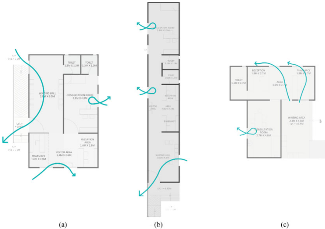
Fig. 17.15 MCs' typologies with different exterior openings in; a R-type, b E-type, and c T-type
