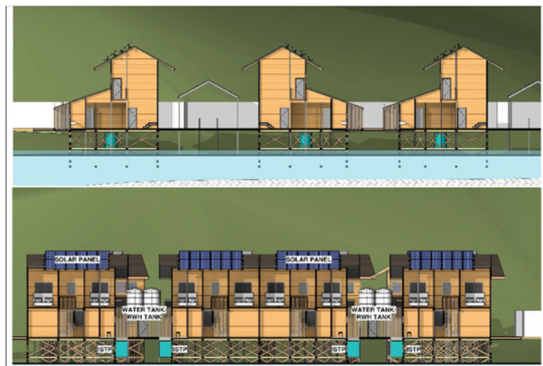
Fig. 4.11 Sectional view across new water village planning model for Lok Urai village, Gaya Island (Illustration by: Nor Efenday)
