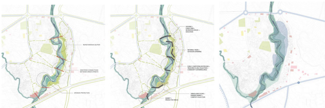
Fig. 3.2 Strategic plan for Kazanchis neighborhood: Connection, Housing, and Flooding. Connection diagram (left): potential bridge connections across the river in red. Housing diagram (center): plans for new hybrid bridges in black, with proposed housing and other amenities. Flooding diagram (right): areas of predominate flooding along the river meander in blue. AARC
